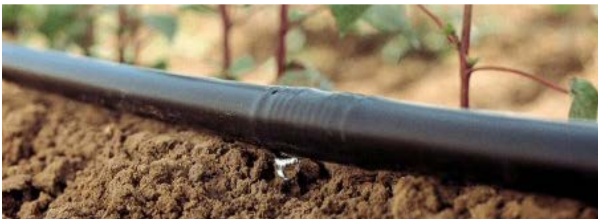
Fig. 21 The right thing: a droplet of water -having almost zero relevant pressure- leaves the dripper
