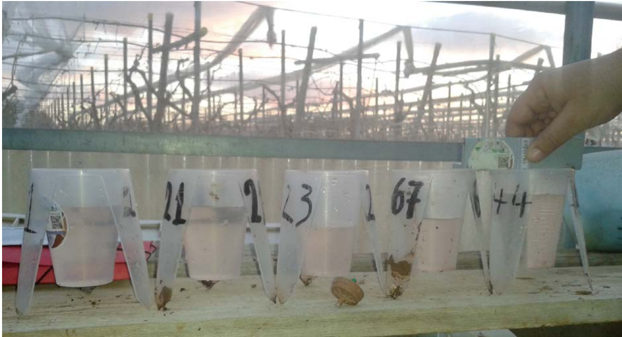
Fig. 26 Catch-cans from a micro-irrigation audit
