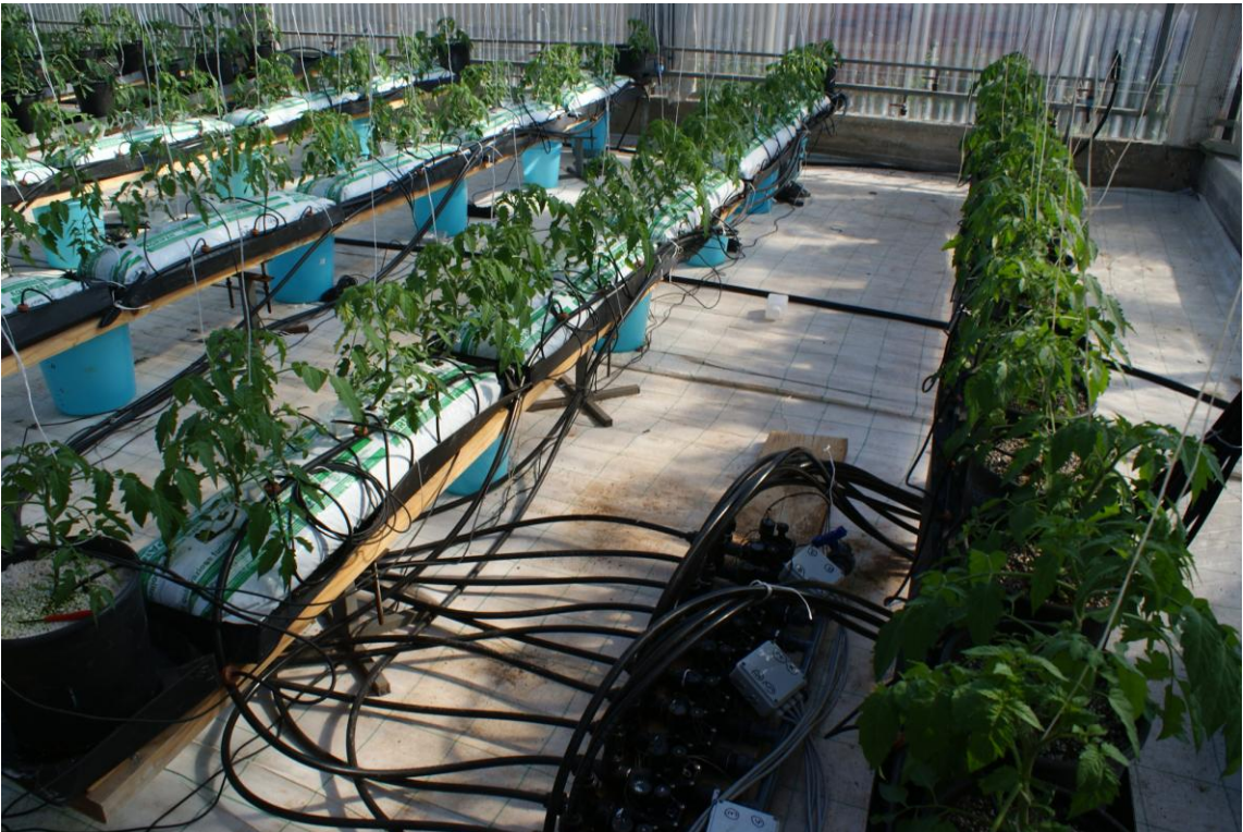
Picture 4-5: Experiment on the use of capacitance soil moisture sensors for assessing the effects of different substrate water content on growth and water relations of soilless tomato
