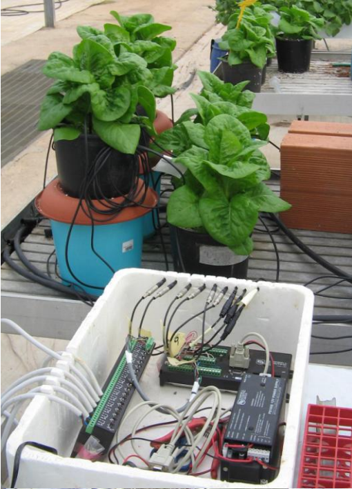
Photo 2-3: Experiment on Timer versus moisture sensor-based irrigation control of soilless lettuce
