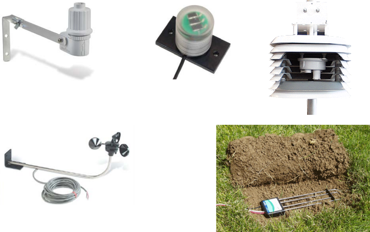
Fig. 11 Sensors (rain, solar energy, air temperature and humidity, wind speed and soil moisture).
