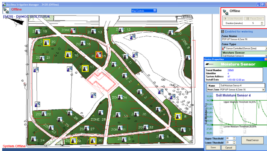
Fig. 10 Screen shot from software for central irrigation control of a landscaping setup
