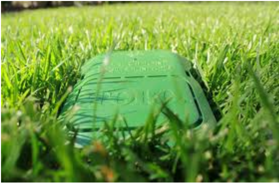
Fig. 25 The receiver (up) and the sensor (down) of the TORO PSS system (the upper photo presents the receivers of the 3 experimental replications: A, B and C, each one of them corresponded to one sensor).
