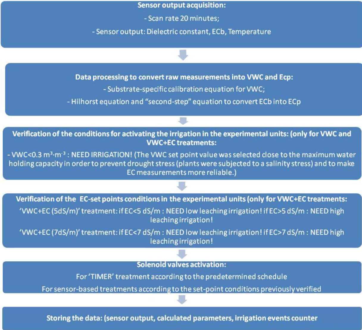
Fig 6: Scheme of the data acquisition and processing algorithm in the program used for the automatic irrigation system.
