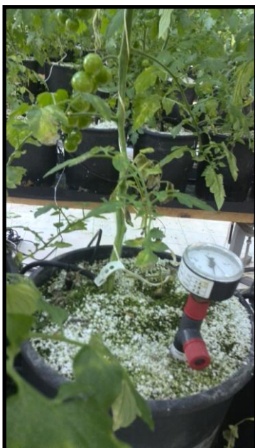
Picture 2: Particular of the pot in the experimental unit containing a tensiometer and a GS3 sensor.
