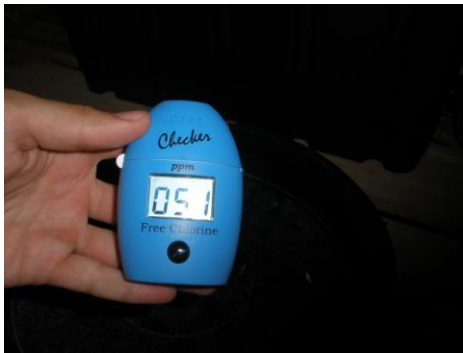
Figure 14 Free chlorine checker
