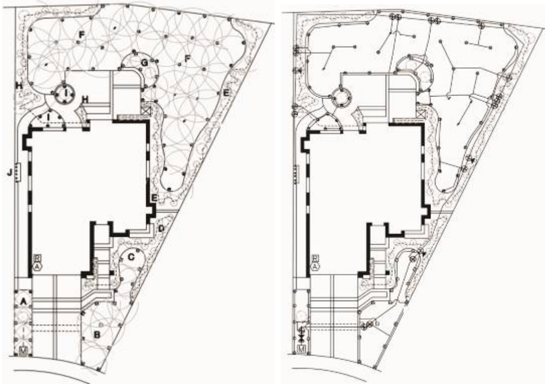
Fig. 63 Irrigation design of landscapes according to the positions of the sprinklers (Rainbird, 2001)
