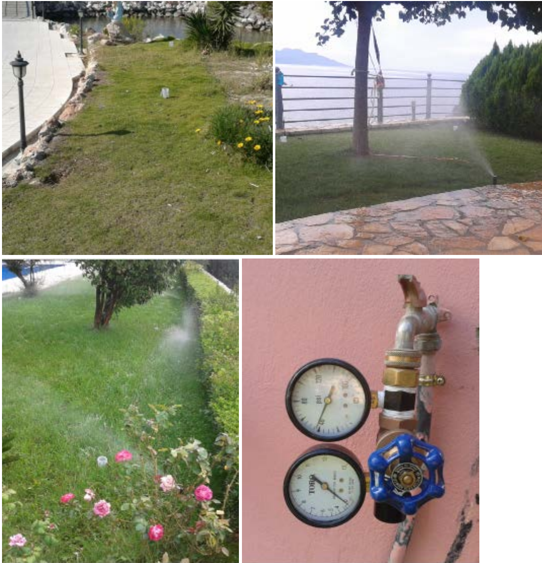
Fig. 66 Catch can test and flow rate - pressure test
