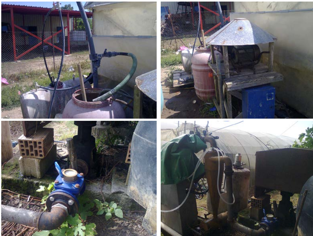
Fig. 51 Hydrocyclone, drill and irrigation fertilizer system in a selected greenhouse
